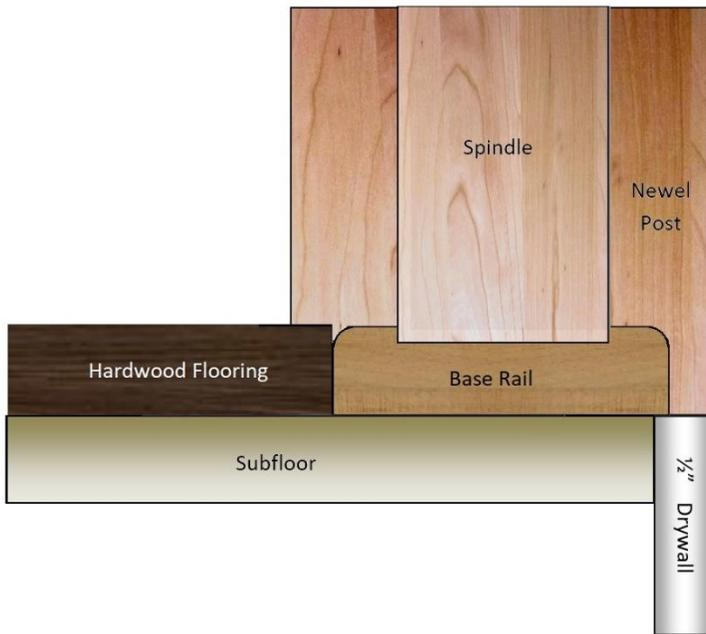
**This is incorrect, when the base rail is installed to the subfloor a number of problems can occur:**
