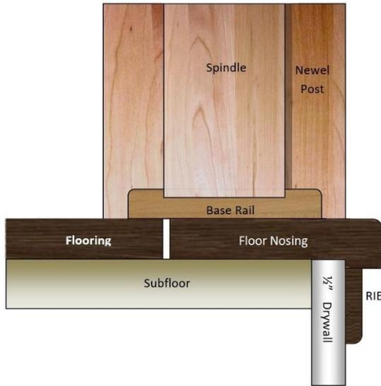
If you are installing a hardwood or laminate your flooring manufacturer might have a matching floor nosing. Install the floor nosing first and fasten the base rail to it. The flooring can be installed at the same time or later, as the base rail will hide any gap between the two pieces. Depending on the style of nosing you may require additional R1E trim to finish the transition and hide any imperfect cuts in the drywall.
