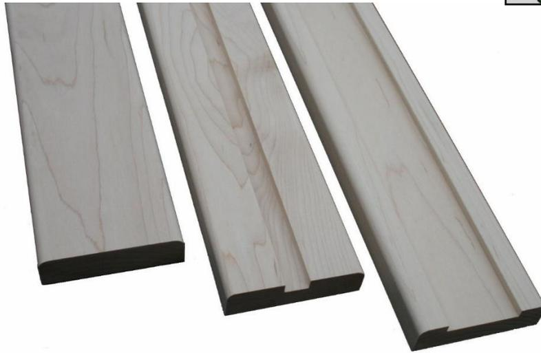
**Base rail is a standard finishing material that the spindles fit into. Typically, the base rail is fastened down using nails or screws that are hidden once the spindles are installed. Our standard base rail measures 2 7/8" x 3/4", manufactured in solid for round spindles or glass clips, 1/2" dado for square metal spindles, and 1 5/8" dado for square wood spindles.**
