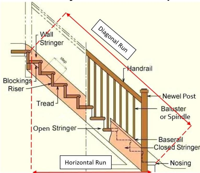
For an open stringer the spindles are installed into the treads. Typical installations require 2 wooden spindles or 3 metal spindles per tread. The spindle at the front of the tread will need a 35", the 1 or 2 spindles on the back of the tread will be at least 42", cut to fit. For a closed stringer the spindles are installed into a base rail on top of the stringer, they will be 35".
