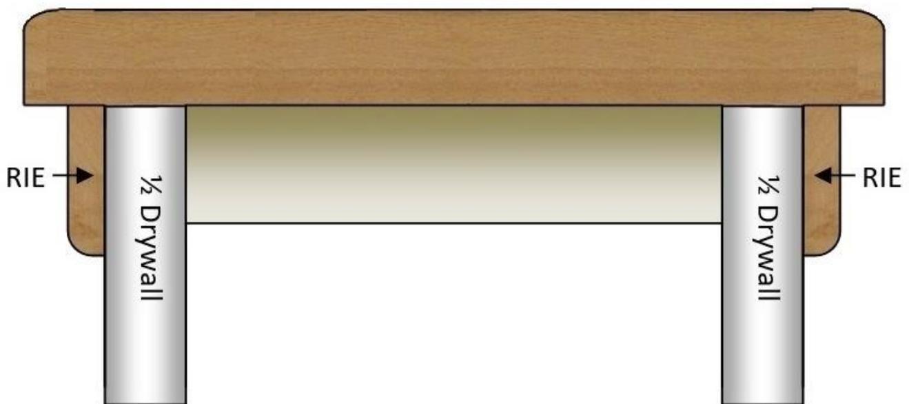
By using a cap piece that is wider than the finished wall you can create a nosing with overhang, a small trim (we use R1E) is fitted underneath to hide the drywall seam. This ensures a clean finish and allows for some human error cutting the drywall.
