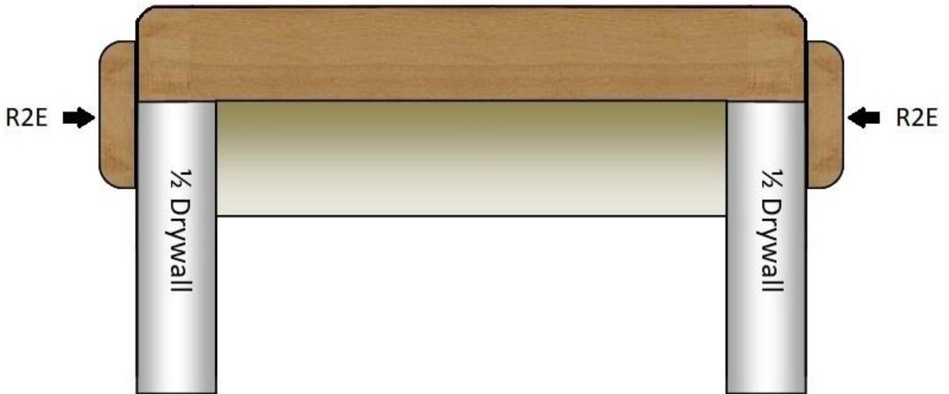
**For a sleeker finish a cap piece the same width as the wall is fitted to match the edge of the drywall. Our slim trim, the R2E is used to cover the seam between the drywall and the cap. The drywall cut does need to be a little more precise as there is less trim to cover the seam. Custom trim can always be made if you need something specific to finish your project.**
