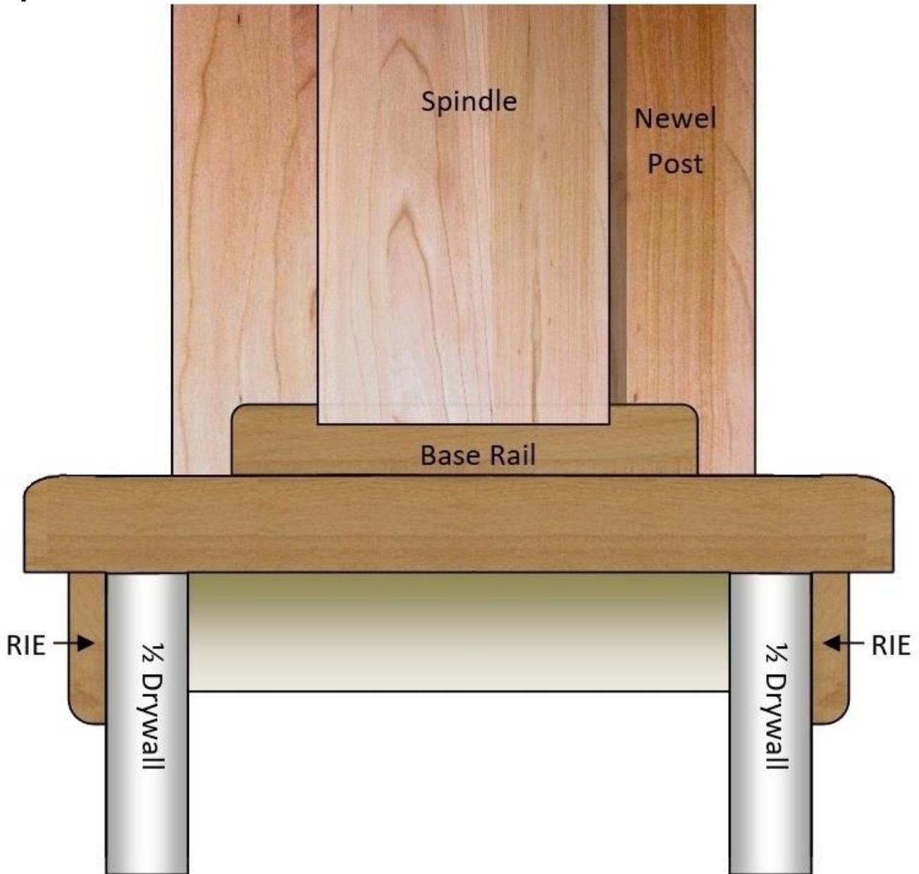
**In a typical installation the post, base rail and handrail would be installed centred on the stringer, creating a balanced symmetrical railing. Of course, not every home is the same and you may need to offset the installation.**
